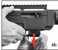
**Figure 4.** The safety should be "on" when the magazine is being removed or inserted. Move the magazine release forward (Figure 4a) and draw the magazine out by grasping it between your thumb and forefinger and draw it out of the gun (Figure 4b).
