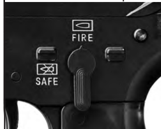
fig. 2 Manual safety in “FIRE” position
