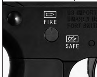
fig. 4 Manual safety in “FIRE” position
